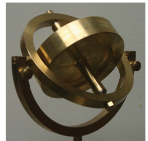
FIG. S1. (left) Coordinate system for the gyroscope. Space axes in the inertial frame are (x, y, z) ; axes in the body frame are (x^*, y^*, z^*) ; and Euler angles that relate the two systems are \theta, \phi, \psi . The intersection of the (x, y) and (x^*, y^*) planes is the line of nodes. (right) In the gyroscope shown in the photograph, z^* is along the spin axis and the line of nodes is the axis of the outer semicircular gimbal ring.
